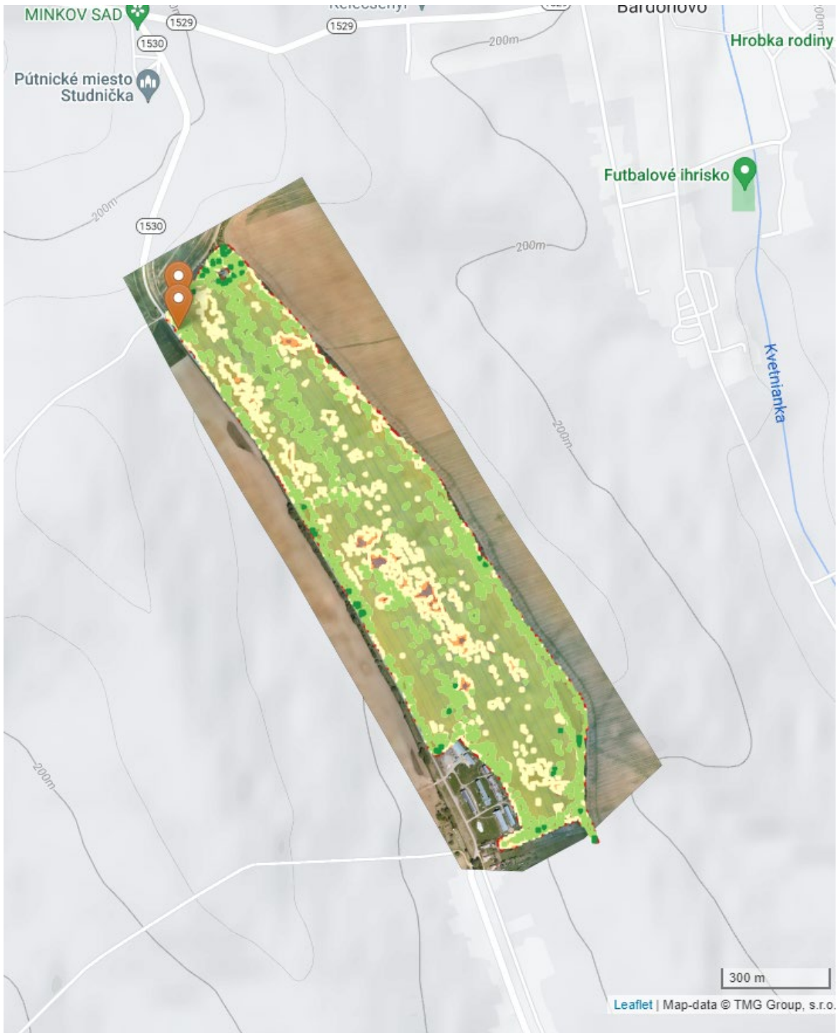
Figure 6: Vectorized NDRE - this can be uploaded into the software of agricultural machines and tractors
